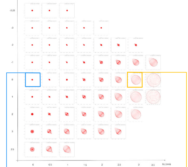
Figure 4. Aberration map in the lens created using the spot diagram map at the min RMS diameter location. Circles containing 50% and 87% of the energy are displayed.
