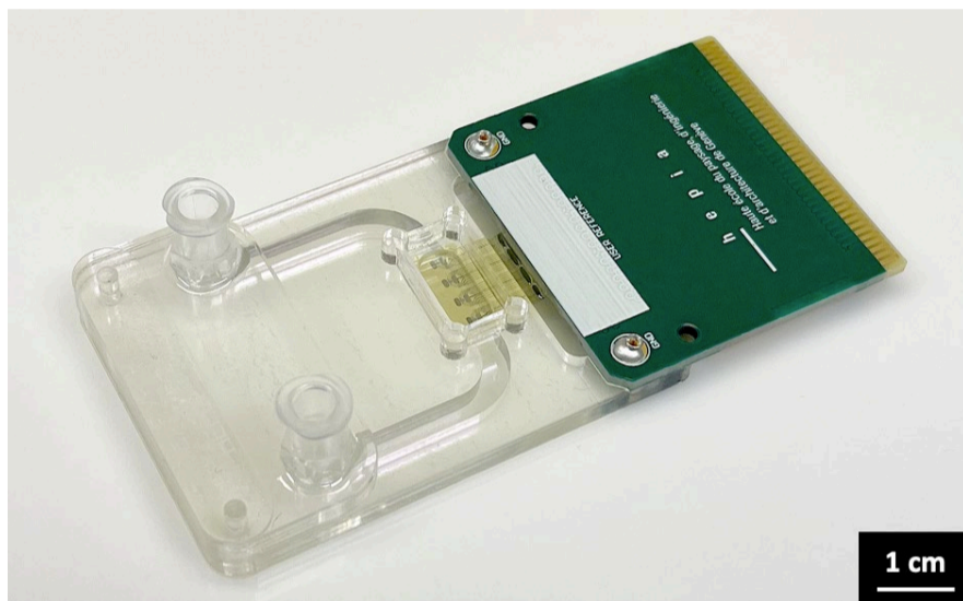
Figure 1: Realised biochip composed of a porous polyimide membrane comprising 4 recording areas with 8 recording sites at each.
