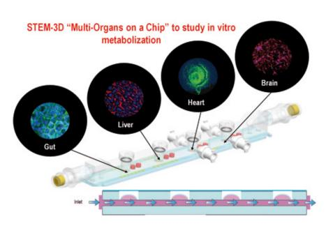
Micro-organs are placed within micro-chambers with bio-sensors connected through a microfludic system.
