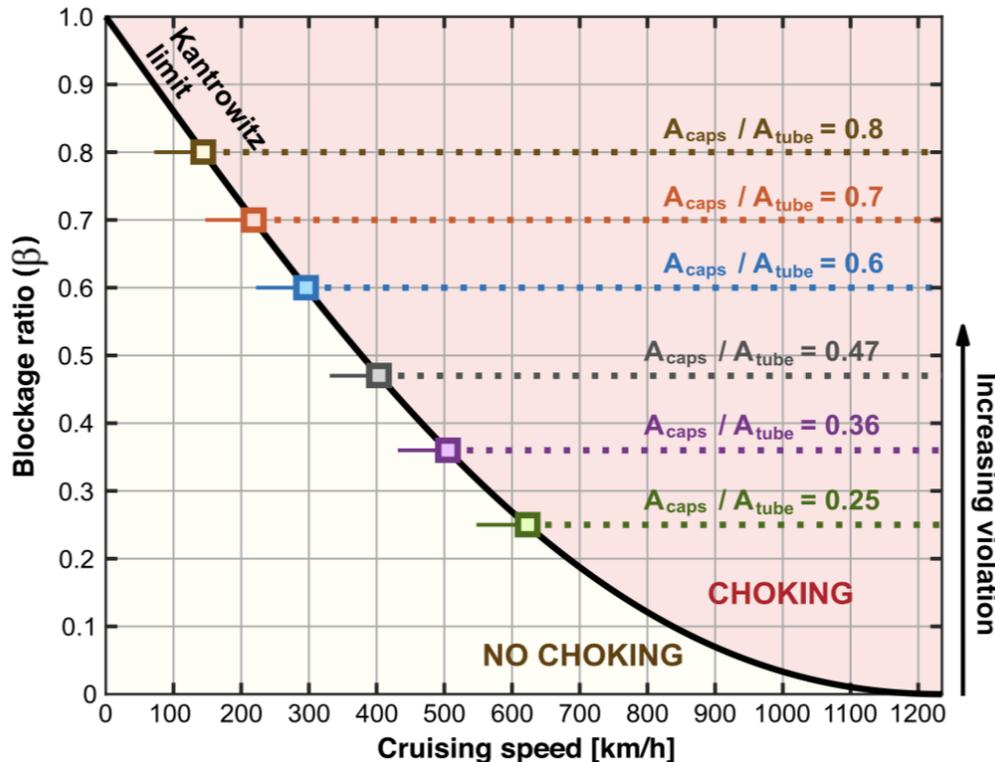
$$\frac{1}{1 - \beta} = \frac{1}{Ma} \left( \frac{1 + \left[ \frac{\gamma - 1}{2} \right] Ma^2}{1 + \left[ \frac{\gamma - 1}{2} \right]} \right)^{\frac{\gamma + 1}{2(\gamma - 1)}}$$
