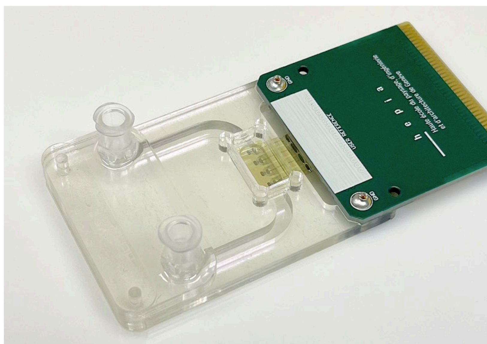
Figure 4 MEA biochip composed of a porous membrane (yellow part of the device) comprising four recording areas with eight electrodes at each.
