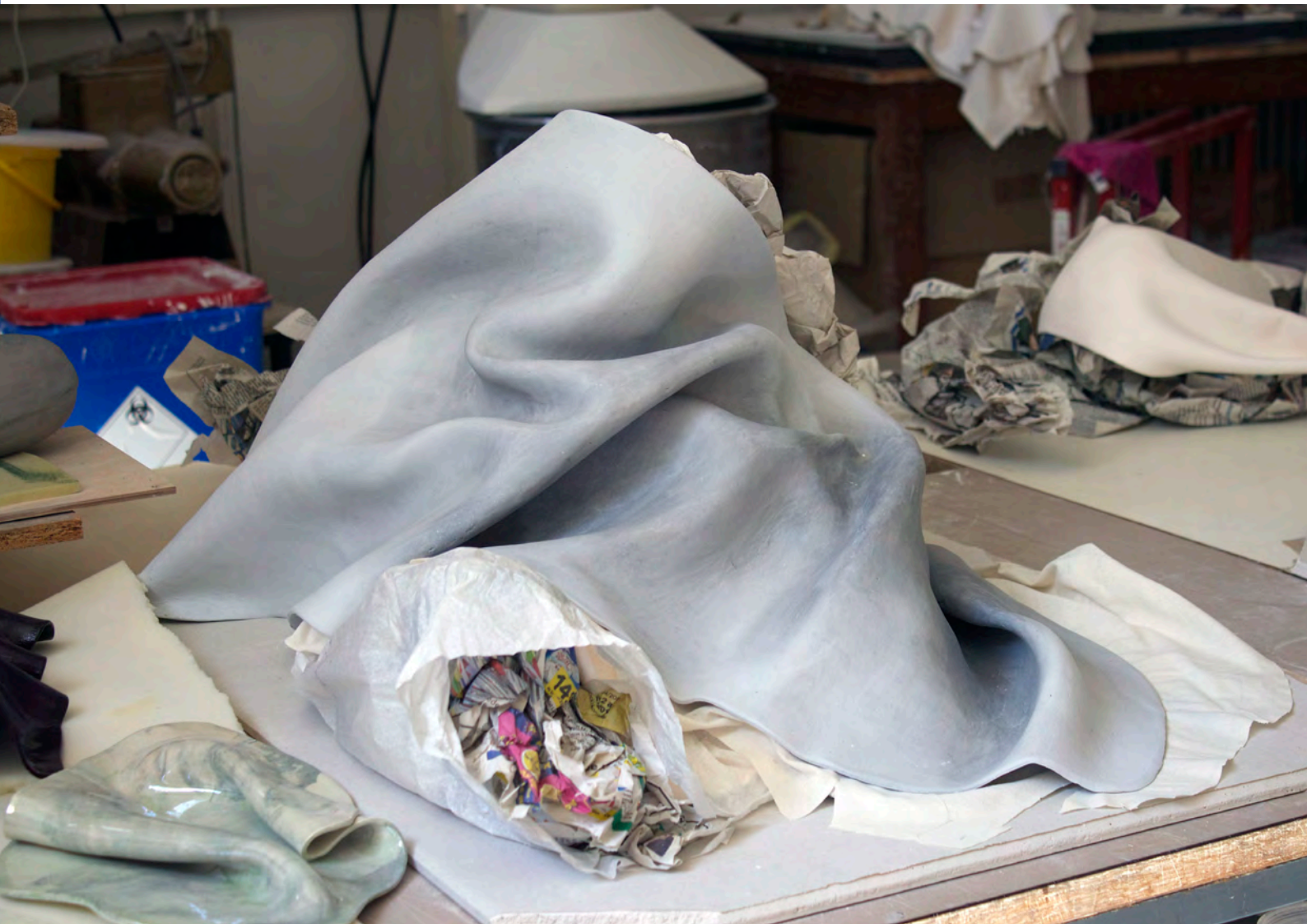
Coloured porcelaine in drying process, unfired
